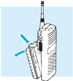
3. Place the battery in the charger pocket with the four silver contacts to the back. Lean the top forward as far as you can to seat the battery properly.
