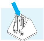
4. Tilt the battery back against the contacts until it snaps into place.
