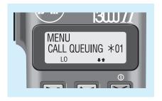
To view details of each call press the Enter  $(\rightarrow)$  key. The call position in the queue and the caller's Selcall identity will be displayed. The first call is always displayed until you scroll through the queue.
