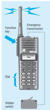
The T3020 II can be set up to make an emergency call to a preprogrammed party (usually your base or despatcher). This facility may be accessible via one of the function keys, or a switch fitted externally to the radio.
