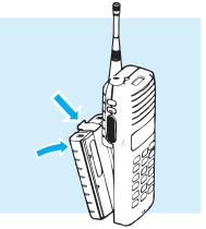
**Note:** When using a trickle charger, recharging the battery pack with the radio attached *and* switched on will reduce the amount of charge the pack receives. To ensure that an exhausted battery pack is completely recharged, it should be charged for a full twelve hour period either separately, or with the radio switched off.
