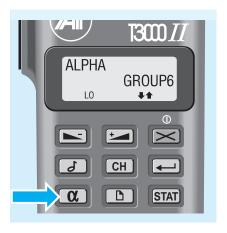
Press the Enter (→) key to initiate the command sequence. If the sequence is a call, this is set up and conducted in the usual way.
