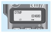
Key in the required DTMF string using the numeric keypad, then press the Enter  $(\leftarrow)$  key to initiate the call. Depending upon how your radio is programmed, the digits may be transmitted separately with each individual key press, or the string may be transmitted in its entirety when the Enter  $(\leftarrow)$  key is pressed.
